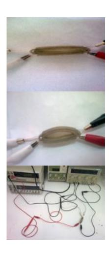
An artificial urinary sphincter made of two-way shape memory NiTi alloy embedded in silicon rubber is designed for prosthesis surgery in case of patients who suffer from urinary incontinence. The metallic part curves down when actuated by electrical current and straightens up when the current stops. This produces a smart composite for urination control in patients inflicted with spinal cord injury.
